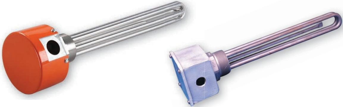
**Over-the-Side heaters** are designed for the robust requirements of corrosive chemicals, viscous (potentially contaminated) fluids, and rinse and process water heating. Various configurations of tubular heater element assemblies provide convenient tank side mounting. As required, heaters are constructed with risers, junction boxes and element support legs.
