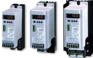
**Durex's SSN DIN rail mount solid state relays (SSR) and SSJ (SSR)** are an excellence solution for switching resistive current loads of up to 35 amps. Designed in a compact size, SSRs with integrated zerocross or phase fired control switching offer superior temperature process control in most applications.
