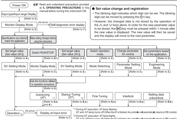
\*3 Adjust the PID constants manually when the optimum PID constants cannot be calculated by AT or ST for characteristic variations of the controlled system
