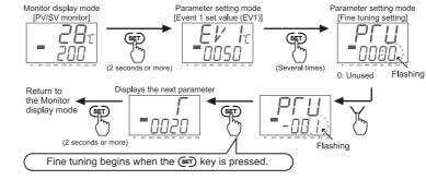
If the set value of Fine tuning is returned to "0: Unused," Fine tuning correction will no longer be applied to control.
