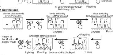
The Set lock level (Lock) settings can be changed after lock is executed.
