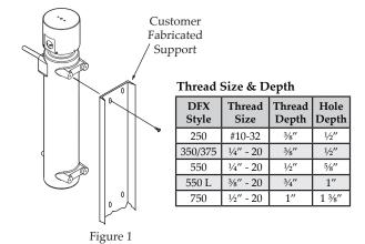
Enclosure "Down" orientation is recommended for higher temperature outlet applications (300°F or 150°C+) to reduce enclosure temperatures. If the heater has a "stand-off" enclosure, mount the heater vertically with the enclosure up.
